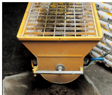
Mixing Mapecem in a mini-batcher
