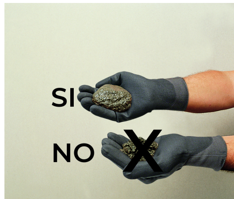
The correct consistency of Mapecem
